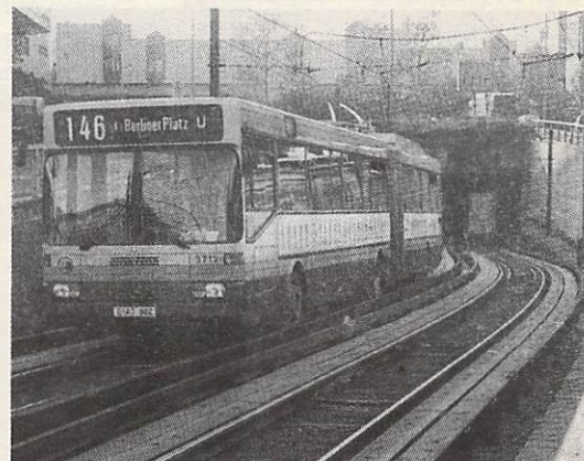
The city of Essen has met the increasing challenge individual transport poses to public transport. The first track-guided bus operation commenced in 1980. Since 1988, these buses have shared the city tram tunnel to avoid city centre traffic chaos. Passengers enjoy a smooth trip to the city without interruptions, past congestions.
